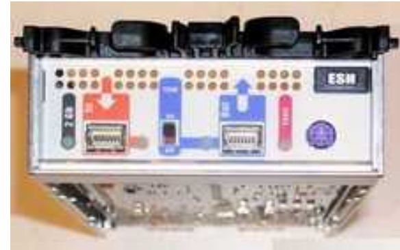
ESH shelf module – notice the termination switch
